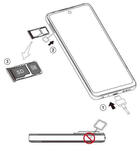
**Caution:** Do not insert the SIM pin into the small hole on top or bottom of the phone.
