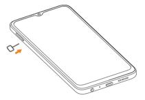
Step 2. Remove the NANO SIM card/microSD card tray.
