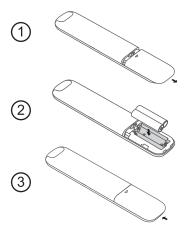
Insert batteries in the correct polarity as indicated in the battery compartment.
